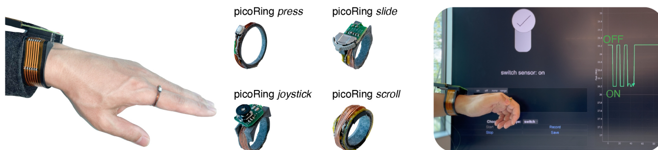
Figure 1: Overview of picoRing. picoRing is a flexible sensing architecture enabling a variety of battery-free smart rings paired with a wristband. This paper shows four types of picoRing that support thumb-to-index finger pressing, sliding, or scrolling.
