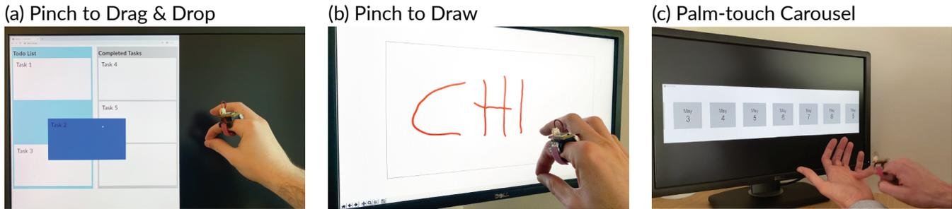
**Figure 7: ElectroRing’s ability to detect subtle touch/release events with precise timing enables a number of useful applications when combined with a pointing technique such as an IMU: (a) In-air drag & drop using finger pinches. (b) Pinch to segment strokes while drawing in mid-air. (c) Carousel/slider with inertia controlled by taps/swipes on the palm.**
