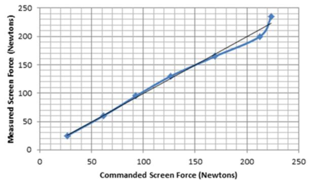
Figure 6. Plot of measured force vs. commanded force.
