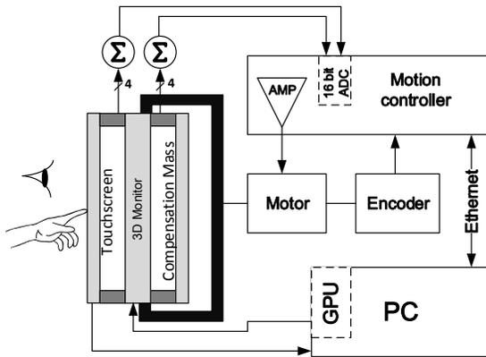
Figure 4. TouchMover system schematic.
