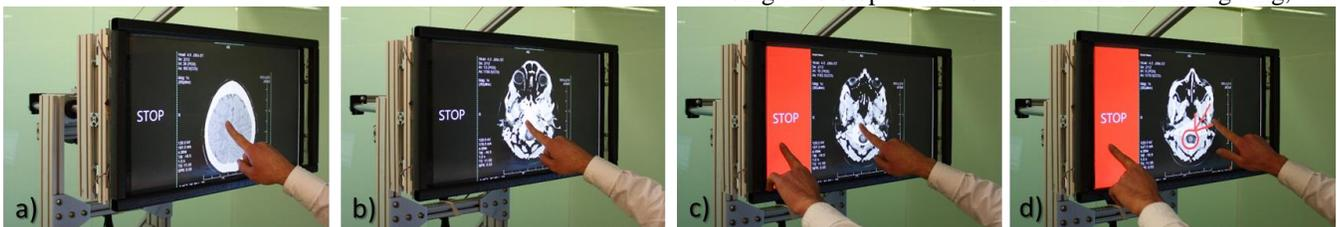
**Figure 8. Interacting with medical volumetric data.** We used the MRI scans of the human brain in our application. Pushing the display back reveals different images of the scan dataset (a-b). The user can prevent the device from moving by touching on a stop button (c) and then annotating the current slice with their finger (d).
