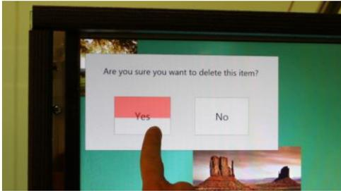
**Figure 10.** An example of touchscreen interactions augmented with kinematic haptics. Z-buttons (e.g., *Yes* confirming deletion) require higher force and larger displacement of the screen than others to eliminate accidental activation. The button rendering serves as a progress bar, visually reinforcing the amount of movement necessary to complete the action.
