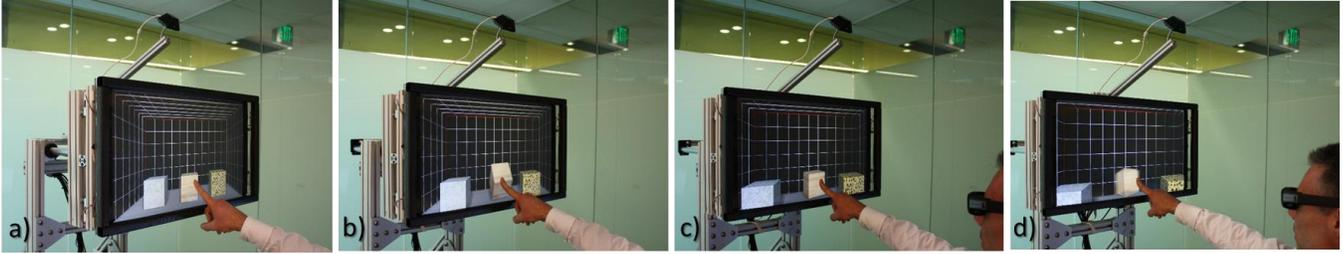
**Figure 7. Application example of a 3D physical simulation with force feedback. By moving the screen with their finger, the user can interact with on-screen 3D objects and experience different force responses that correspond to the physical simulation. Note: stereo is absent from figure for clarity.**
