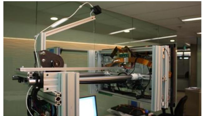
Figure 3. Image of the back side of our device showing the rack and pinion gear and the completely supported 3D touchscreen up front (consult Figure 2 for explanation of the components).
