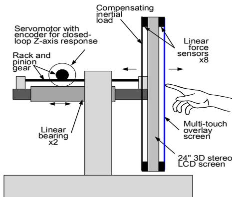
Figure 2. Simple diagram outlining major components of the TouchMover device.
