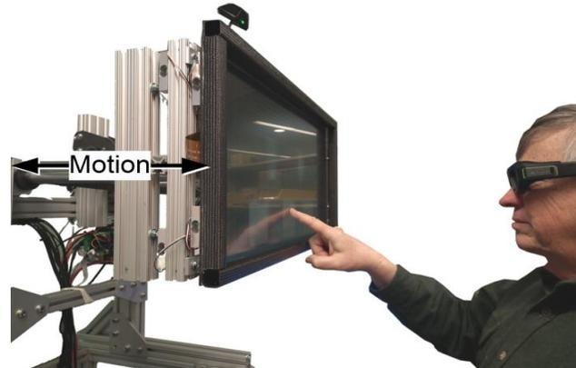
**Figure 1. TouchMover co-locates immersive 3D stereo visualization, direct touch and touch force sensing with a robotically actuated display.**
