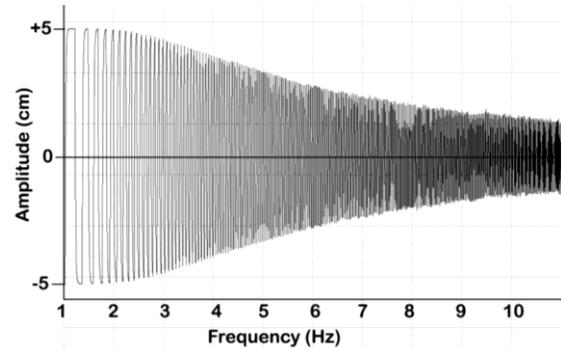
Figure 5. Bode plot of movement amplitude vs. frequency.
