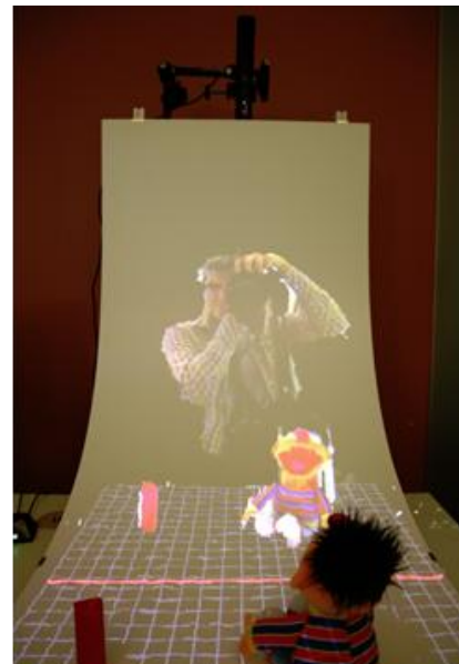
Figure 4. Mirror view of real-time captured data of the user and the objects on the tabletop (stereo projection is disabled in this picture for clarity). Note that, even though the screen curves, the 3D captured data as well as the grid which represents the tabletop surface appears correct from the user's perspective.
