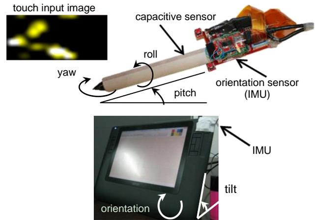
Figure 1. Pen and tablet augmented with sensors.
