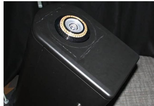
Figure 3. The projector-camera unit with a wide angle lens and the infrared illumination ring around it.
