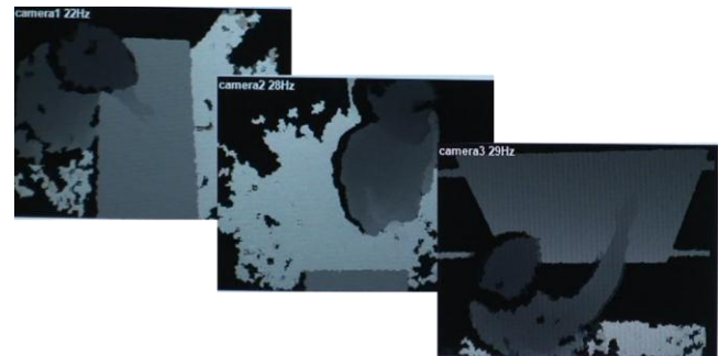
Figure 8: Raw depth images collected from three depth cameras each capturing a different part of the scene. Except where black, pixel intensity is proportional to the distance to camera (depth).
