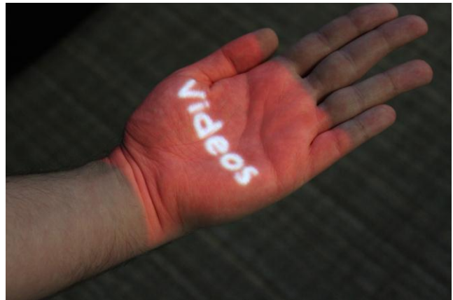
Figure 10: By aligning the projectors and the cameras, we can correctly project virtual content registered with the real world. In this case, we project a menu option directly onto the user's hand.
