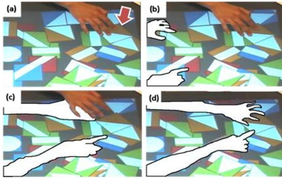
**Figure 6.** This sequence illustrates how the arm shadows helped users avoid conflict. Lasting 2s, we see (a) the local user manipulating a tile; (b) a remote user’s arm shadow approaches from the left; (c) the remote user arrives, and the local user begins to withdraw his hand; (d) finally, only the remote user is manipulating the tile. For print legibility, we have traced the arm shadow and made it opaque.
