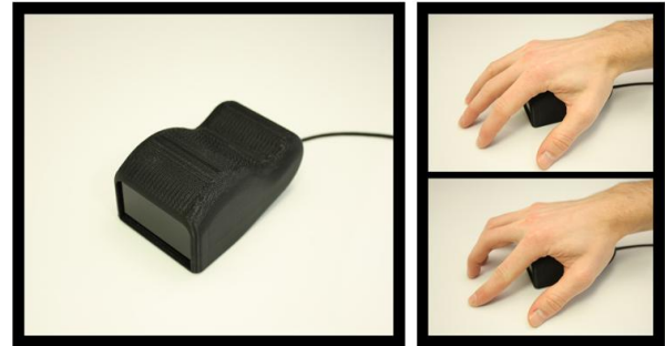
Figure 10. Side Mouse rests under the palm of hand, allowing fingers to touch the table surface directly in front of the device. These are sensed using an internal camera and IR laser.
