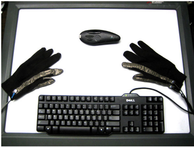
Figure 5: Interaction devices used in our experiment (top to bottom): A 3DOF tracked three button wand (Logitech TrackMan Live), a pair of specially constructed gloves with two active fingers on each hand, and the keyboard. The devices are laid out on the DiamondTouch surface.
