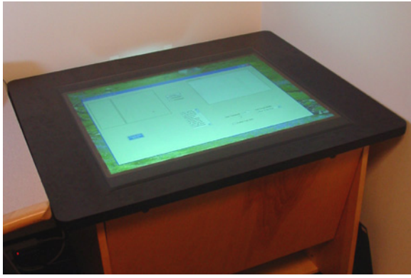
Figure 9. Our multi-touch back-projected tabletop display prototype uses an infra-red illuminant and camera to detect contacts through a diffuse surface.
