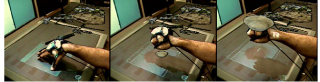
Figure 1: Frames from a cross-dimensional pull gesture implemented in VITA. (left) Selecting a 2D object and starting to form a grabbing gesture. (middle) The 3D object appears from the table. (right) Holding the 3D object. (Table is covered with black paper to provide a darker background for imaging the projected display through the live tracked video see-through display.)
