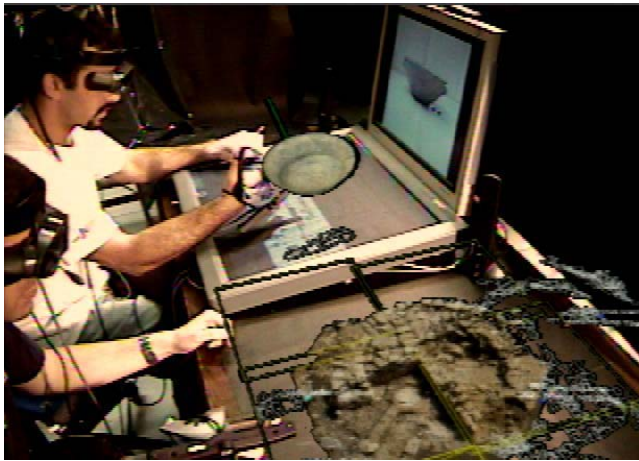
Figure 2: Two users, wearing tracked, see-through, head-worn displays and tracked 3D gloves, interact with 2D and 3D objects in VITA.
