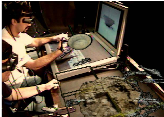
Figure 2: Two users, wearing tracked, see-through, head-worn displays and 3D gloves, interact in VITA.
