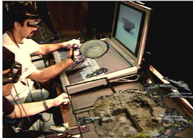
Figure 1. Two users simultaneously collaborate in VITA. While one user is inspecting the 3D virtual model of the ceramic vessel above the table comparing it with the high resolution image on the screen, the second user is looking at the 3D miniature terrain model next to the table. (Video see-through capture).
